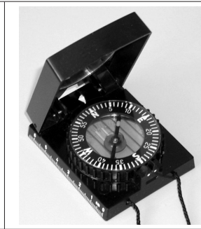
Figure 3. East German compass with a mirror. Photo by Stefan Kühn
