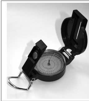
Figure 2. Liquid-filled compass. Photo by Zbigniew Podgórski
